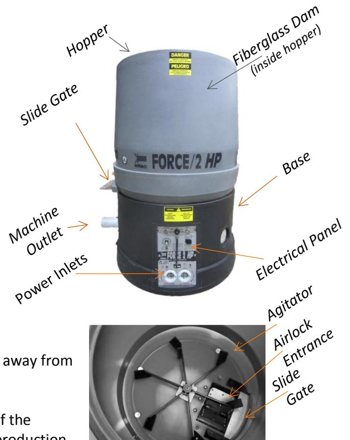
**Airlock:** The airlock transfers the insulation from the agitation system into the airstream. Note insulation does not come into contact with the blower. Insulation is discharged from the airlock by way of the machine outlet into the hose. Hose is not shown in above diagram; hose is connected to the Machine Outlet.
