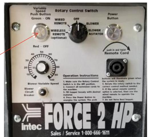
*Note 1: If you desire to use the blower's variable speed, place this switch in the 'ON' position. Then, set the variable speed dial to the desired setting based on desired blower speed.*
