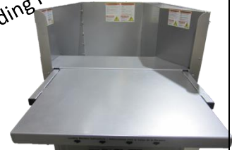
Hopper holds volumes of insulation
