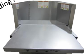
Hopper holds volumes of insulation
