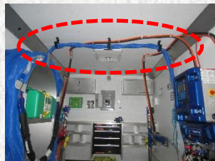
Description: Spray Foam Hose Hooks. Used on ceiling to allow spray hose to span from reactor to hose hood with ease in removing hose when beneficial.
