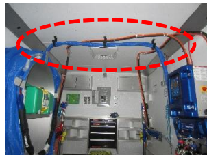
Part #'s: 77081-10 Description: Spray Foam Hose Hooks. Used on ceiling to allow spray hose to span from reactor to hose hood with ease in removing hose when beneficial.
