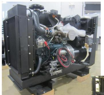
**Powered by Kubota V2403 Turbo Diesel**
